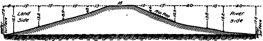
FIG. 108.—Sny levee—section across old channel, known as the cut-off, public road on the crown.
