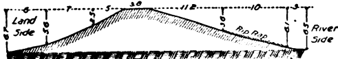
FIG. 97.—Flint Creek-Iowa River levee—section exposed to waves, protected by riprap, has never failed.
