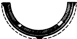
Fig. 58.—Strainer covered with copper wire and gauze.
